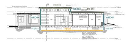
The entire home will be encapsulated and sealed to below 1.0 ACH50. The main level is a full ranch, but there is an attached Accessory Dwelling Unit, which is a basement garden level space. It is accessible from its own entrance outside, or via stairs inside.
