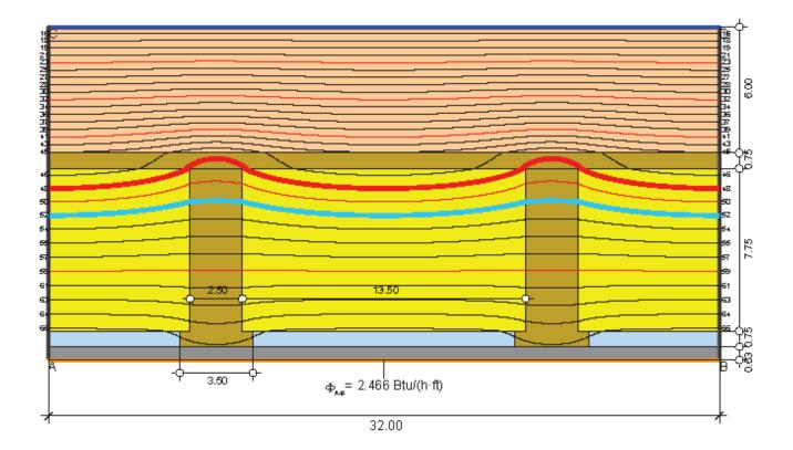
$$U_{m,ke} = \frac{2.371}{30.000 \cdot 0.813} = 0.0972 \text{ W/(m}^2 \text{ K}) = 0.0171 \text{ Btu/(h·ft}^2 \text{ F})$$
