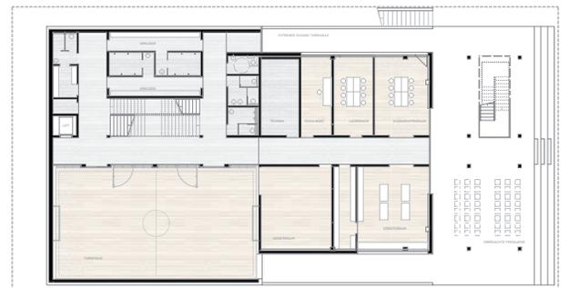
Ground floor plan | Grundriss Erdgeschoss
