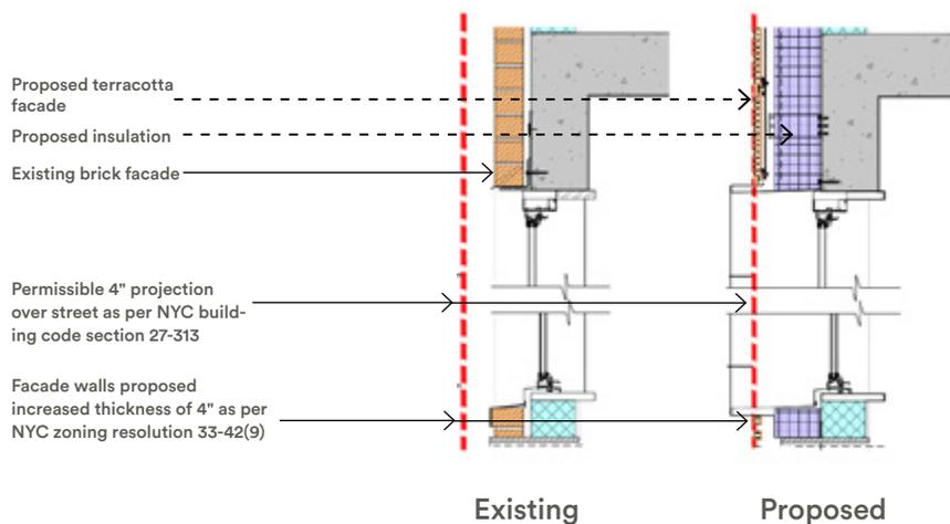
Driven in part by expensive Local Law 11 inspection and maintenance requirements, a 1960's, 142,000 SF, 200-unit, multifamily building in Midtown, is planning to replace its brick facade. Using a zoning code provision, Allen + Killcoyne Architects has designed a passive upgrade to the facade, adding insulation and improved windows to all 16 stories. This will also allow for an overhaul and reduction of the buildings mechanical system.
